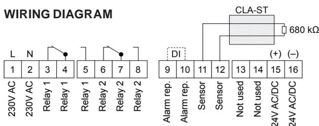
The relay outputs are shown in alarm/no power on condition. Max 5A, 250V
